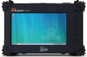
The **eo TufTab® a7230XD** features a unique WACOM® dual-mode screen that automatically switches between resistive touch screen and active digitizer (pen) input.
